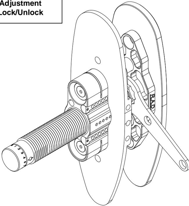
To unlock the pad adjustment use the 5/8 wrench supplied with the unit to loose the Adjuster Screw. Position the pad to the desired location and retighten.
